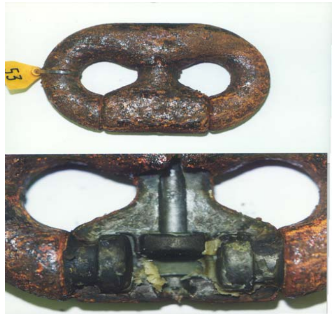
E-2000-Protected Samples after 150 cycles, Closed (top) and Open (bottom)
